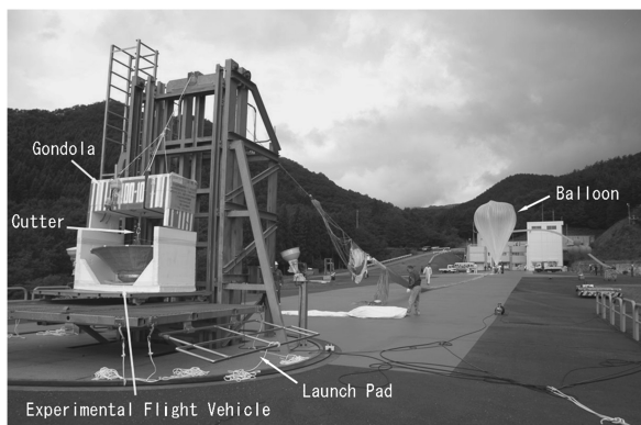
Fig. 7 Experimental flight vehicle with the gondola on the launch pad before launch.
